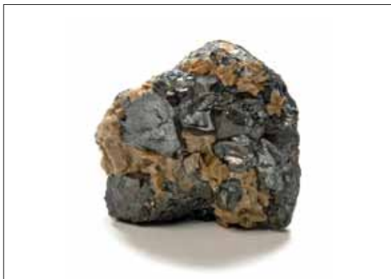
Slika / Figure 3. Tetraedrit sa sideritom, Maškara, Gornji Vakuf, BiH / Tetrahedrite with siderite, Maškara, Gornji Vakuf, B&H (prema / after: Operta 2009).
