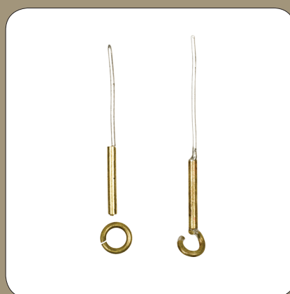
Lotanje alkica i žice (stanjene na kraju). Brazing loops and wire (tapered at the end).
