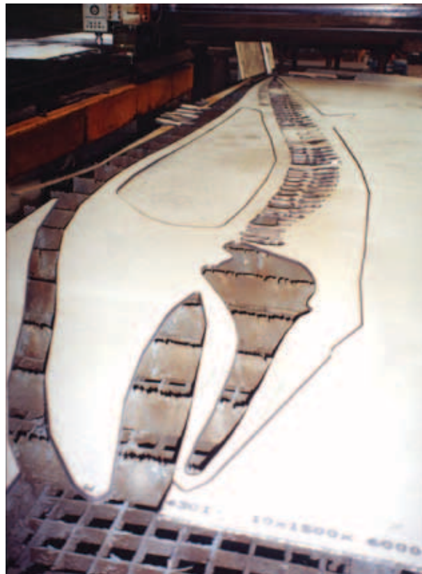
Izrezivanje konture kita iz inox lima Cutting out the contours of a Whale from inox sheet metal
