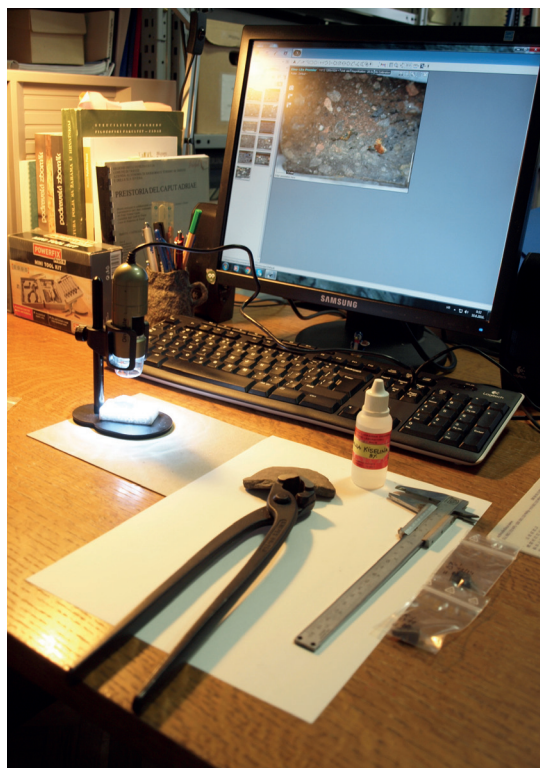
Slika / Figure 1. Digitalni mikroskop spojen s računalom i oprema potrebna za rad: kliješta, pomično mjerilo, zip-vrećice, otopina solne kiseline, keramički uzorci i sitni alat (snimila: A. Kudelić). / Digital microscope connected to a computer, and the equipment necessary for work: pliers, caliper, zip-lock bags, hydrochloric acid solution, pottery samples, and small tools (photo by: A. Kudelić).
