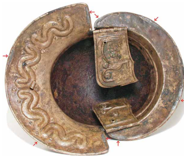
Slika 11 – Raspored vidljivog lema na obrubnim trakama Fig. 11 – Disposition of visible solder on edge reinforcements
