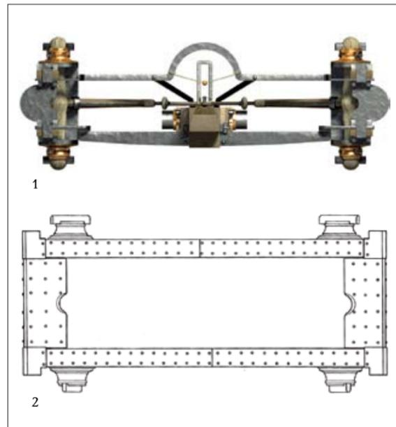
Fig. 17: 1 - The Elenovo spring-frame; 2 - The Hatra spring-frame.
