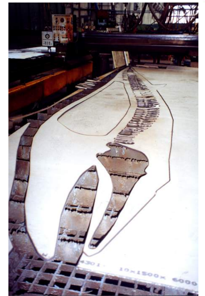
Izrezivanje konture kita iz inox lima Cutting out the contours of a Whale from inox sheet metal
