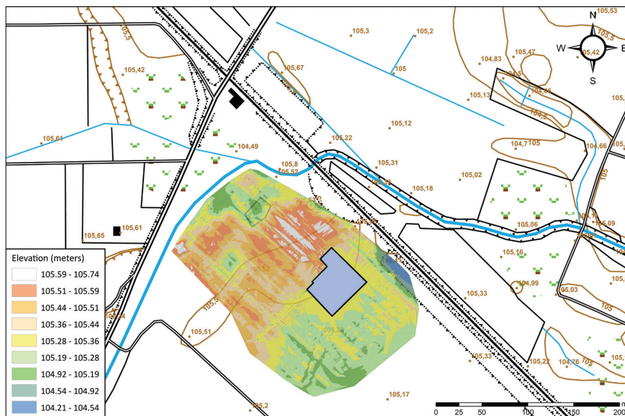
Figure 4: DEM derived from terrestrial topographic survey (author: D. Tresić Pavičić; background after: HOK, DGU).
